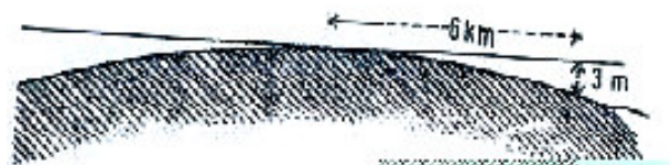
Figure B2 Curvature of the Earth is about 3 m in 6 Km.
